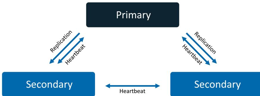
The heartbeat time frame can be tuned, depending on system latency. It is also possible to setup the Mongo DB replica to allow reads from secondary to improve read capacity.
